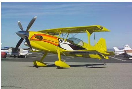
Turbo Tucan. Thrust to weight ratio of 1.5:1.
